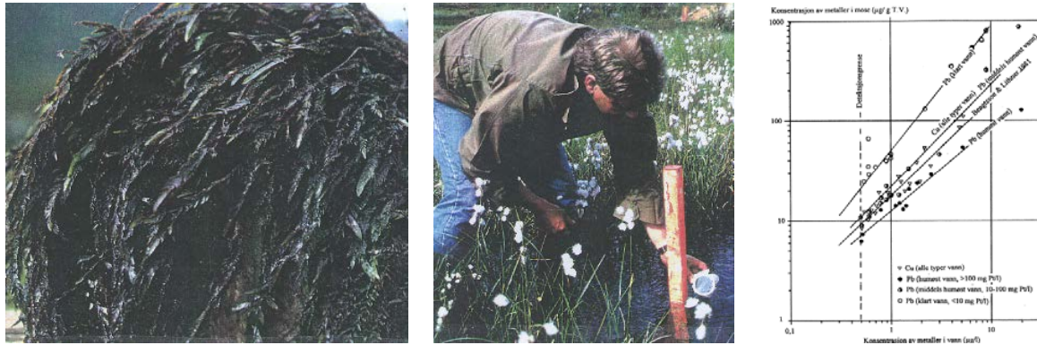
Figure 2: Moss bioindicator Fontinalis antipyretica (left), physical sampling (middle) and reported correlations (right) between concentrations of Cu and Pb in moss and water in the early years of sampling program (Rognerud, 1994).
